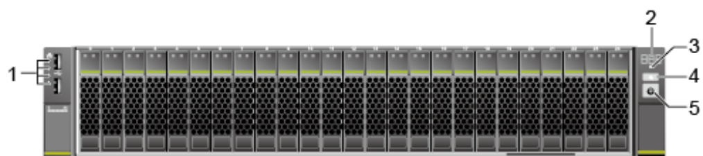
Figure 4-13 Front panel of a server with twenty-five 2.5-inch drives
